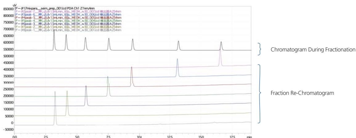
Results of a Purity Check of the Chromatogram During Fractionation and the Recovered Fraction
